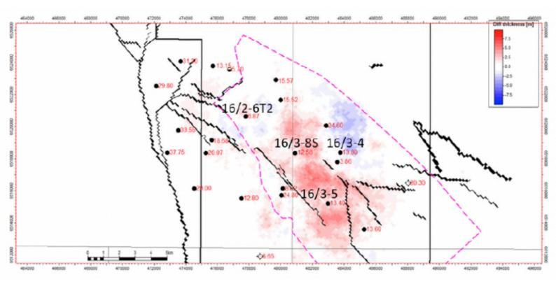
Median of the difference in sand thickness for the initial 200 ensemble members and the updated set conditioned to DST data
