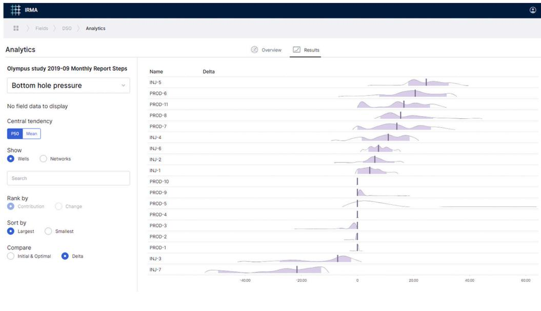
The drainage strategy optimization solution identifies six high-risk/low-value targets on the Olympus field. Exploring an alternative scenario where these six targets are not drilled shows a significant value increase compared with the reactive control (base) strategy.
